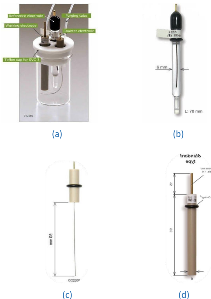
Figure 2: From left to right (a) SVC-3 Voltammetry Cell (b) Reference electrode (Ag/AgCl) (c) Counter electrode (Pt Wire) (d) Working electrode (Glassy Carbon).
