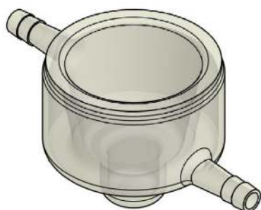
Pyrex cell with thermostatic jacket 430/TJ (Ø9mm thermostat piping)
