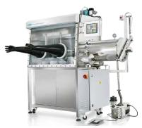
This single workstation system is equipped with an integrated gas purification system (one column), PLC controller (with a touchscreen HMI), electronics enclosure, large and small antechambers, replaceable sight glass, and vacuum pump. Attainable purity of this system is H2O < 1ppm, O2 < 1ppm.
